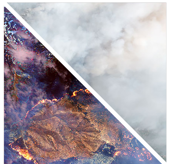
SWIR data can be used for thermal detection and to penetrate smoke and haze.
